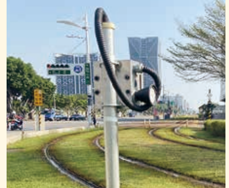
輕軌降噪系統現場安裝 Light Rail Transit Noise Reduction System On-site Installation
