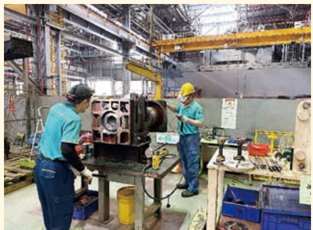
推進馬達拆卸作業 Propulsion motor disassembly
