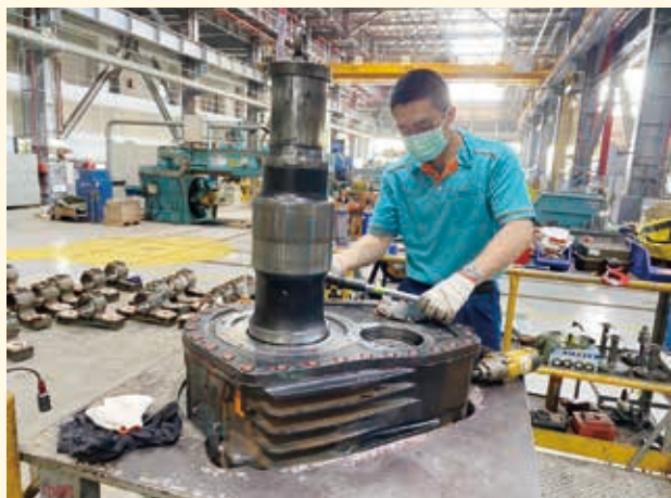
齒輪箱大修 Gearbox Overhaul
