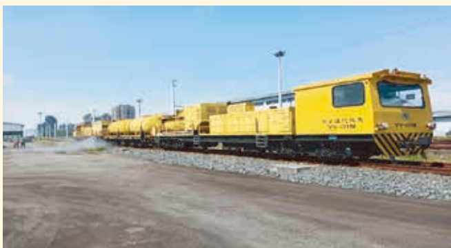
高鐵六家基地清洗車組清洗功能驗證 THSR Liujia Depot cleaning unit cleaning function verification
