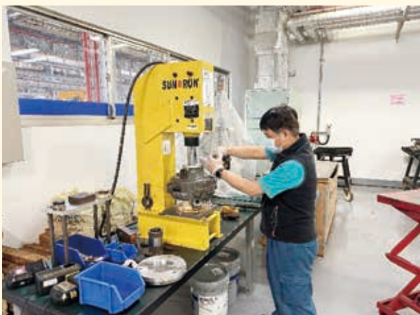
煞車缸翻修作業 Brake cylinder refurbishment
