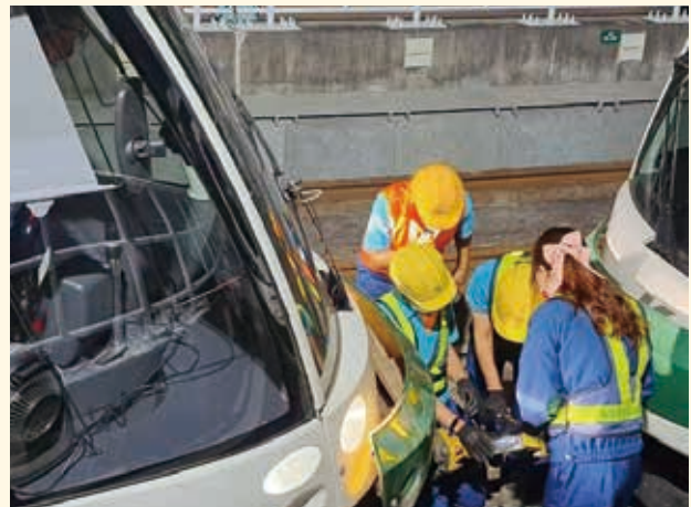
事故車與支援車開始進行聯結 Accident car and support car begin linking
