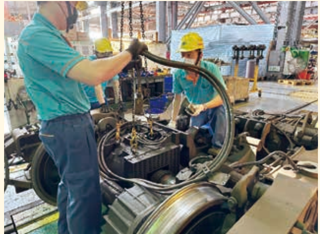
轉向架組裝作業 Bogie Assembly
