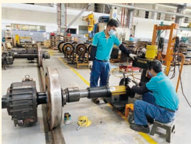
頸軸承組裝 Neck Bearing Assembly
