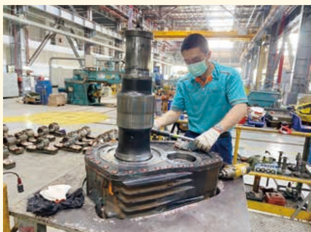
齒輪箱大修 Gearbox Overhaul
