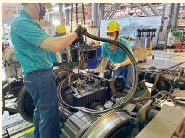
轉向架組裝作業 Bogie Assembly
