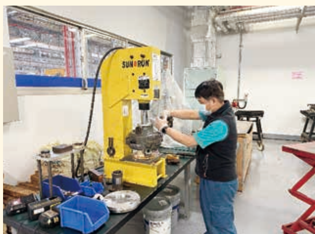
煞車缸翻修作業 Brake cylinder refurbishment
