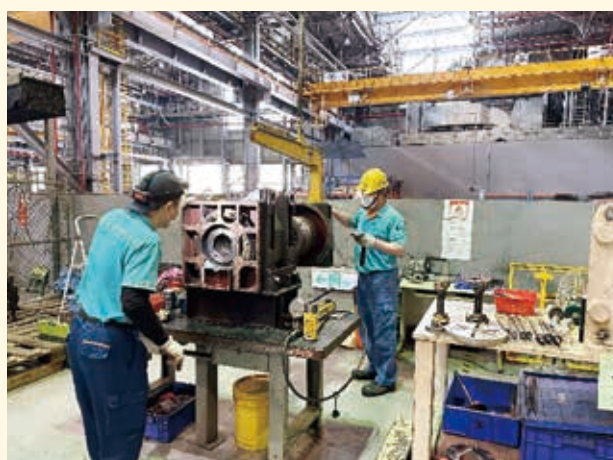
推進馬達拆卸作業 Propulsion motor disassembly
